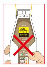
3. Keep the optical receiver clean and use cleaning oil when testing bare fiber to achieve the best performance.
