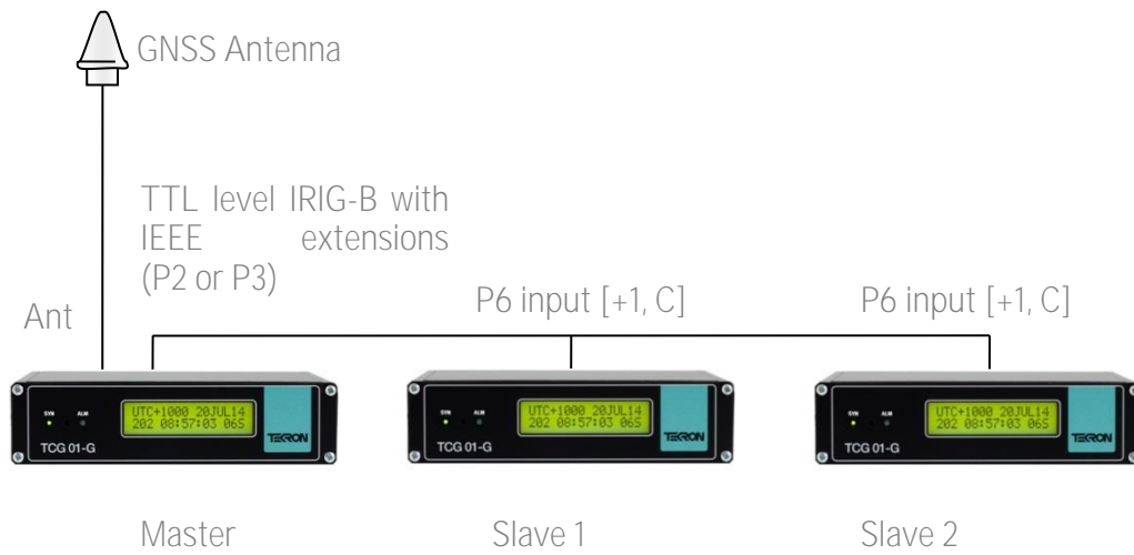
Figure 10 – Multiple Time Code Generators with one GNSS antenna
