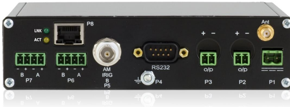
Figure 5 – Rear panel of TCG 01-G, configured with 2-pin connectors (P2 and P3)
